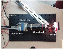
Figure 1. Optical camera setup.
